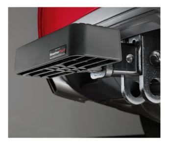
Back out the BumpStep<sup>®</sup> to allow space only for the ball of the foot to rest centered on the the step surface.
