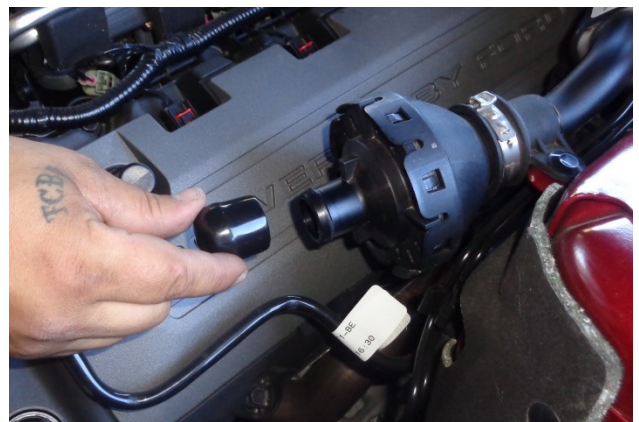
17. Push the vinyl cap (11) onto the resonator.
